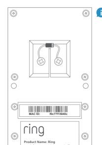
The lighter band on your diode should be on the same side as the wire that runs to the "Front" terminal on your bell.
